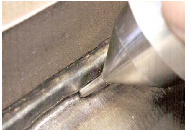
Fig 2 Ultrasonic Peening treatment of Class F fatigue test specimen
